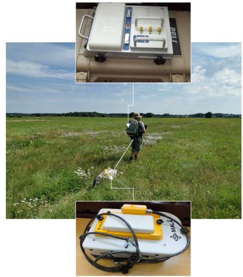
500 MHZ SHIELDED ANTENNA USED DURING GPR SURVEYS (FOT. S. CHWAŁEK)
